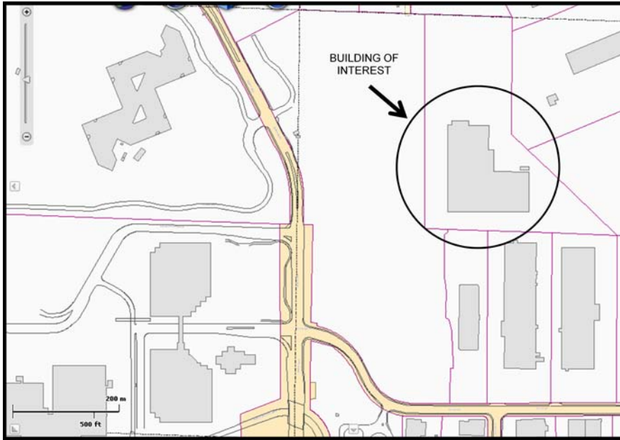
Figure 2. Wide angle view of GIS base map showing a target building, exposures, and roadways. Fire service layers may be on, but viewing them requires zooming closer.
