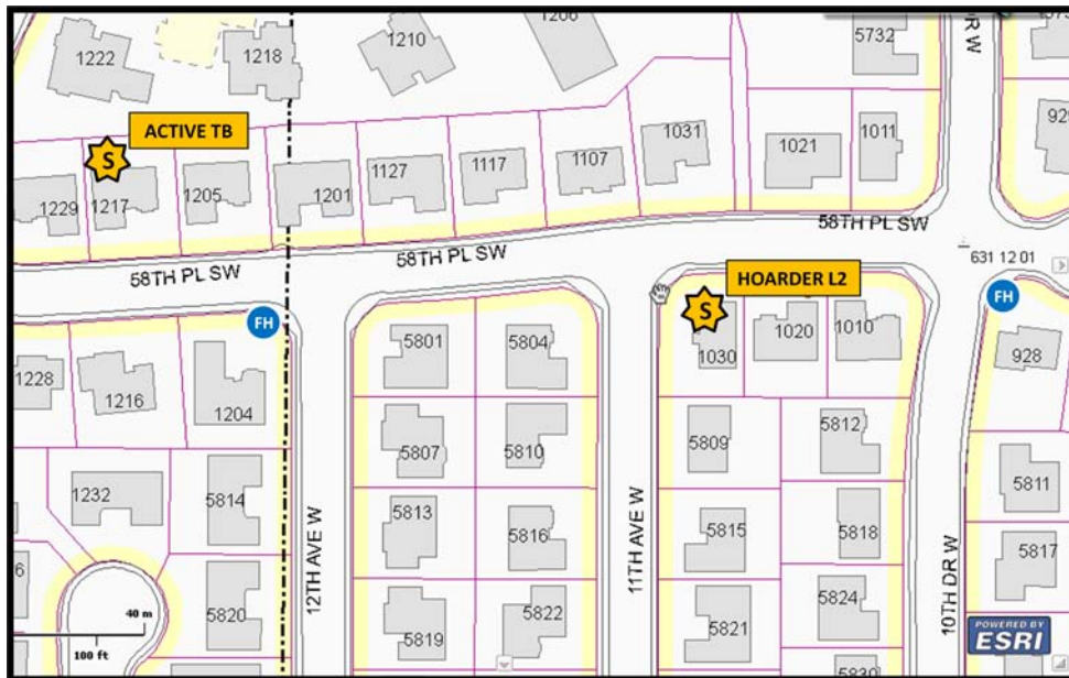
Figure 5. GIS base map of residential neighborhood with special hazards and water supply layers.
