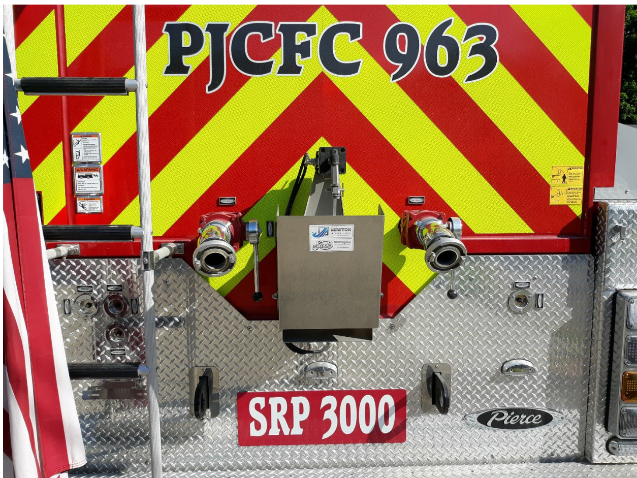
Figure 4. New apparatus with poly tank but no warning labels.
