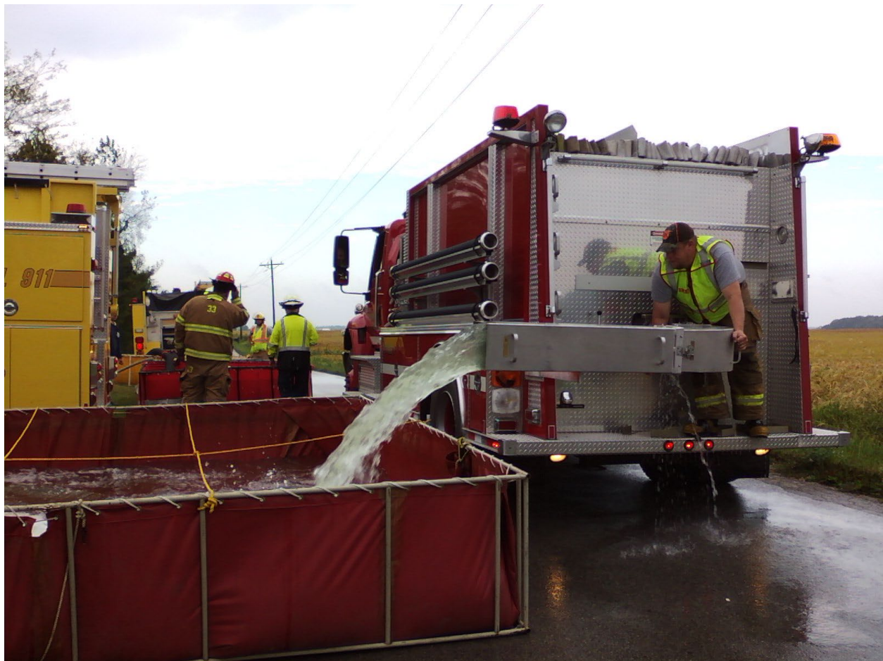
Figure 10. Water tender with adapter to allow side dumping.
