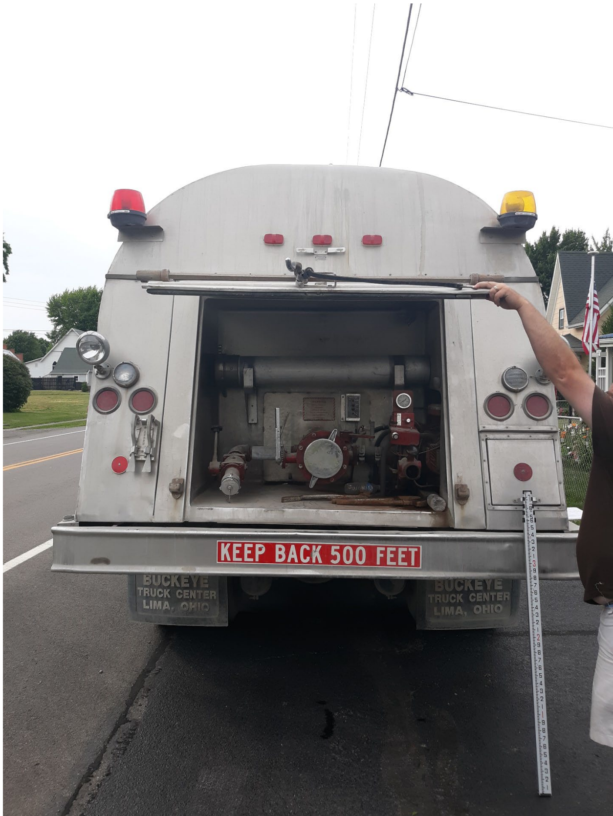
Figure 35. Water tender conversion from dairy tanker.
