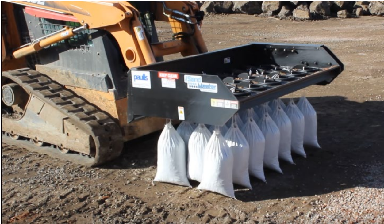
Figure 9. Commercial sandbag filling machine. Retrieved from https://www.equipmentworld.com/video-genius-loader-attachment-can-fill-thousands-of-sandbags-a-day/
