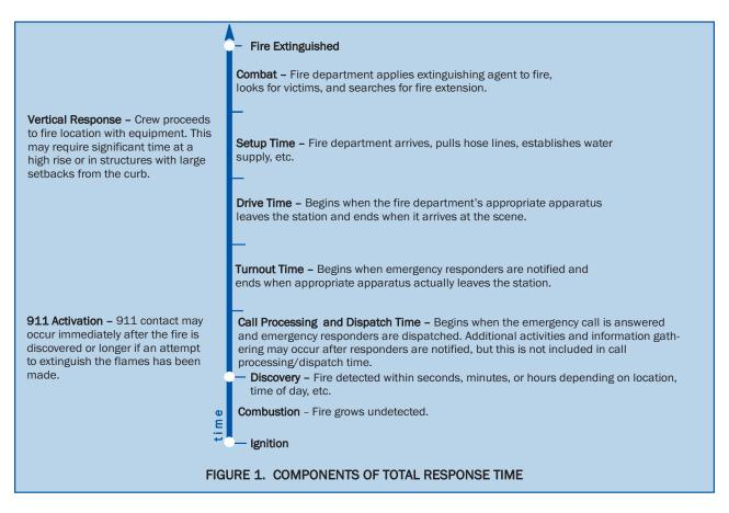
Setup time begins once a fire engine or other apparatus arrives on the scene and ends after personnel established a water supply, set up necessary equipment, etc. Additional time may be required if the structure is set far back from the curb or in a high-rise where a vertical response is required.
