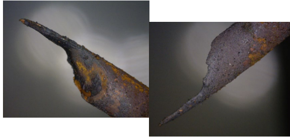
Wire from nonenergized receptacle.
