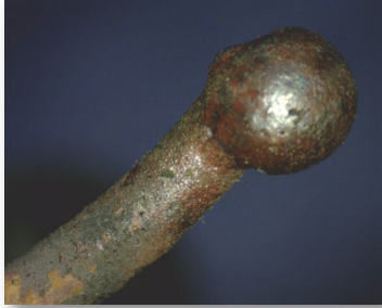
Wire from nonenergized receptacle.
