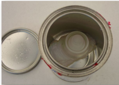
Liquid in plastic container, which dissolved.
