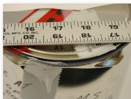
Friction lid seal damaged from stepping on lid to close it — not airtight.
