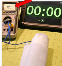
Benchtop test of curling iron wrapped in lightweight combustibles. Time vs. Temperature
