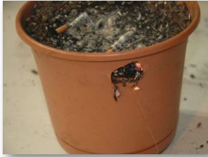
Example: The potential ignition source is the cigarette. What is the first fuel ignited?
