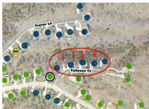
Figure 5: Five homes on Talleson Court were destroyed (red circled). These homes were located at the top of a slope and each had overhanging decks. One home suffered minor damage (blue circled).
