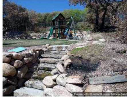
Figure 17: Damage to the play structure slide resulting from radiant heat exposure from the burning Courtney Drive home. Deformation of plastic components (slide and roof) was observed. Scorch or charring of wood structural support members was not observed. Source: IBHS.
