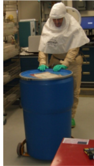
EXHIBIT 11 Ensemble Being Evaluated for Overall Function by Test Subject Moving 55-Gallon Drum. (Courtesy of Intertek Testing Services.)
