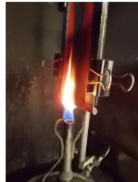
EXHIBIT 10 Exposure of Ensemble Material in Flame Resistance Test. (Courtesy of International Personnel Protection, Inc.)
